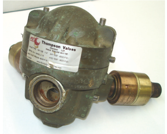
Typical condition before servicing.
